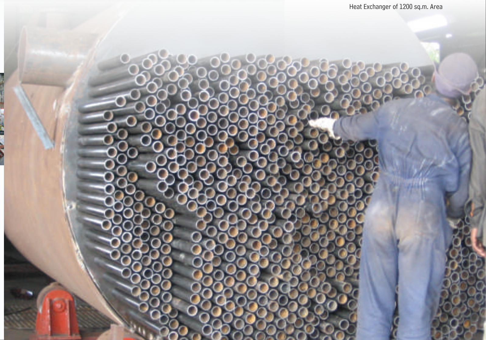
Heat Exchanger of 1200 sq.m. Area
